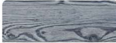
b-Tao: On water-based covering black paint, low-residue white patina paint is applied, and after the drying process is completed, it is cleared using high-grit sandpaper to achieve a special color.
