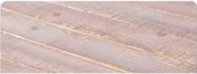
d-Sotka-Çanakkale-Boztepe-Kingo-Hunter (Box): We apply a mixture that we create using our unique techniques to the wooden surfaces of the products and let it sit for approximately 24 hours. This mixture reacts with the extractive substances found particularly in needle-leaved trees, creating a color similar to UV degradation. This color is not a pigment but entirely unique to itself. The tone of the color varies depending on the density of extractive substances within the wood, resulting in shades of brown, green, and gray. It truly provides an aged wood appearance.
